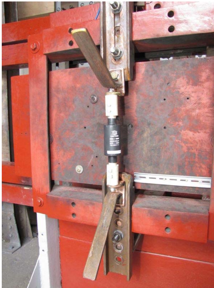
Photo 2: Test arrangement with fuse THS 400
